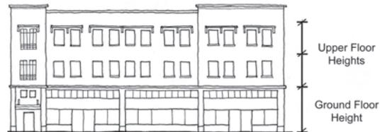
Figure 3.A.18: Floor-to-ceiling heights at the ground-floor should be taller than upper floors.
