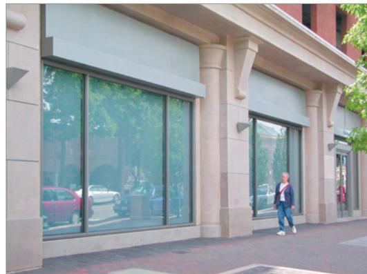
Figure 3.A.35: (Example of Poor Design) Banks often close blinds for security reasons creating blank walls at the ground floor.
