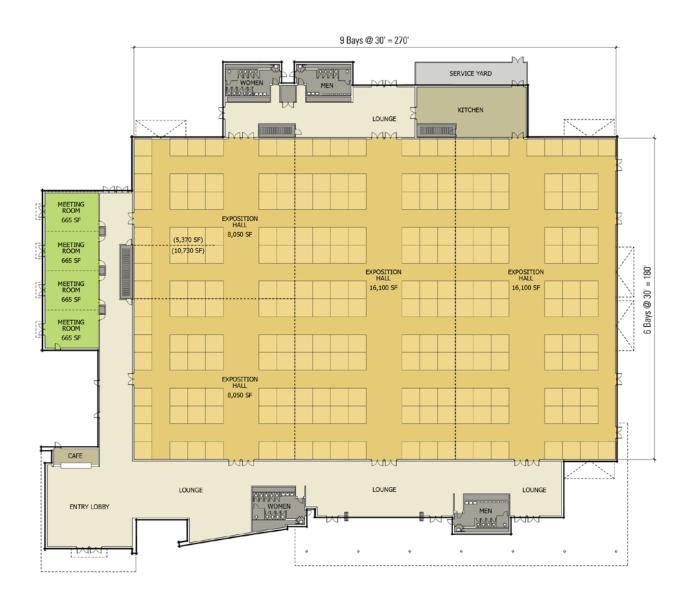
Figure 4.15: Exposition Hall – Schematic Floor Plan
