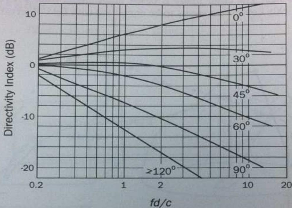
**Figure 9.25** Exhaust stack directivity information based on an experimental model investigation. The quantity  $d$  is the diameter of the stack,  $f$  is the center band frequency in one-third octaves, and  $c$  ( $343 \text{ m s}^{-1}$ ) is the speed of sound in the exhaust gas at the stack exit. The indicated angle is measured from the centerline of the duct.
