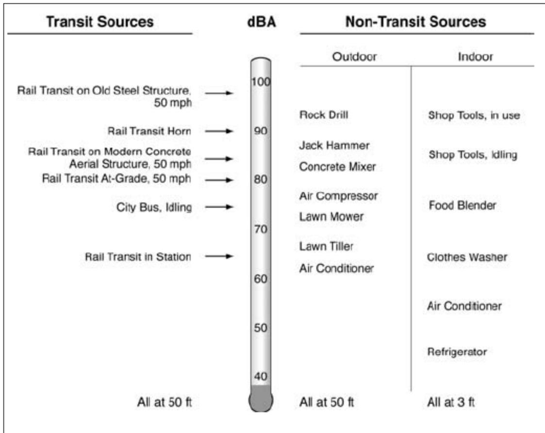
Figure 2 Level of Typical Common Sounds on the dB(A) Scale – (FTA Noise & Vibration Manual, 2006)
